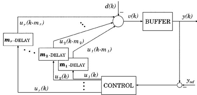
Fig. 1. Dynamic model for the congestion control of ISPNs.
