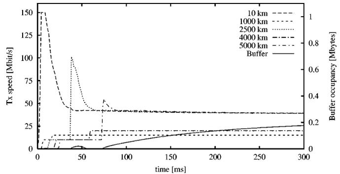
Fig. 6. Transmission rate and bottleneck buffer size. PID controller with five connections at different distances; two are PCR limited.
