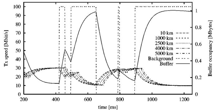
Fig. 7. Transmission rate and bottleneck buffer size. PID controller with five connections at different distances and ON-OFF background traffic.
