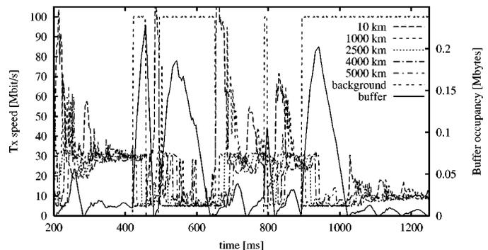
Fig. 8. Transmission rate and bottleneck buffer size. ERICA+ controller with five connections at different distances and ON-OFF background traffic.
