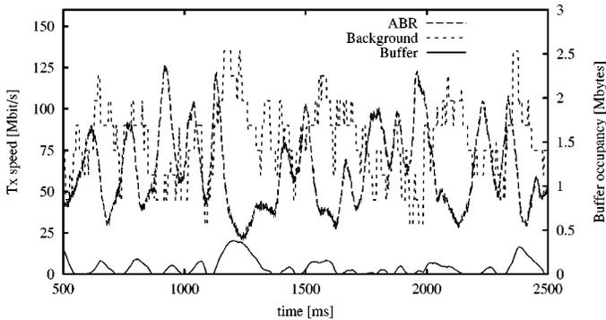
Fig. 10. Total transmission rate and bottleneck buffer size. ERICA+ controller with 100 connections at different distances and ten ON-OFF background superimposed sources.
