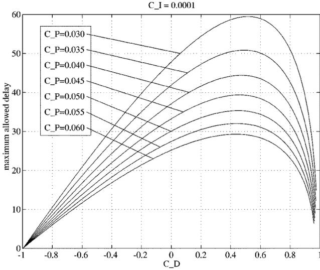
Fig. 3. Value of the maximum allowed delay  $M$  versus  $C_D$  for  $C_I = 0.0001$  and different values of  $C_P$ .
