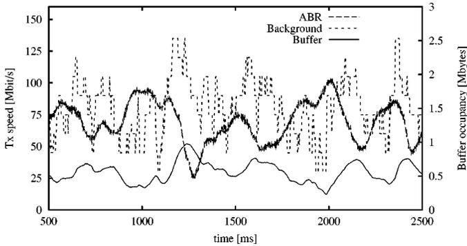
Fig. 9. Total transmission rate and bottleneck buffer size. PID controller with 100 connections at different distances and ten ON-OFF background superimposed sources.
