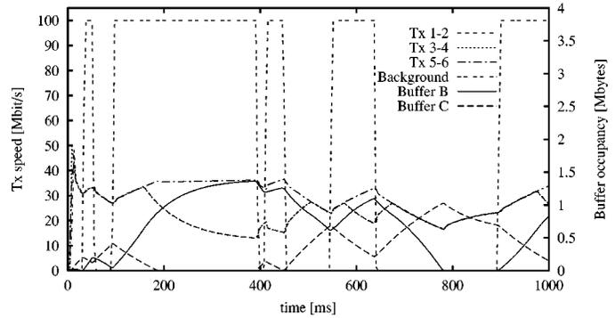
Fig. 12. Parking-lot topology. Transmission rate of the six connections and buffer level at node B and C with ON-OFF background between nodes B and C.
