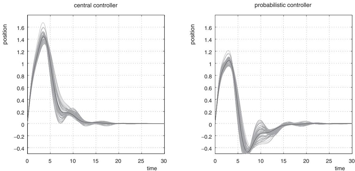
Figure 4. Impulse responses on the soft channel for randomly chosen values of the uncertainty. Central controller (left) and randomized controller (right). The randomized controller is optimized for the average squared  $\ell_2$  norm of the response. Darker lines represent the nominal responses (i.e. with  $\Delta$  set to zero).
