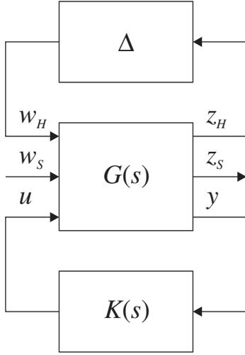
Figure 2. Extended plant with hard and soft performance channels.
