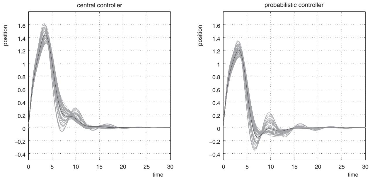
Figure 3. Impulse responses on the soft channel for randomly chosen values of the uncertainty. Central controller (left) and randomized controller (right). The randomized controller is optimized for the average  $\ell_1$  norm of the response. Darker lines represent the nominal responses (i.e. with  $\Delta$  set to zero).
