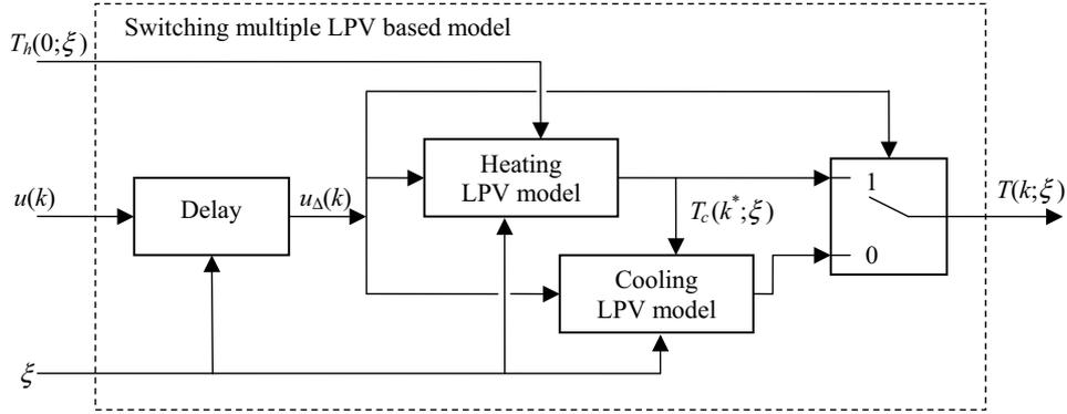
Fig. 2. The switching linear parameter varying (LPV) model:  $u(k)$ , binary valve command signal;  $\xi$ , soil depth;  $u_{\Delta}(k)$ , delayed input signal;  $T_h(0; \xi)$ , initial soil temperature at depth  $\xi$ ;  $T_c(k^*; \xi)$ , soil temperature at the switching instant  $k^*$  at depth  $\xi$ ;  $T(k; \xi)$ , output of the model (estimated temperature of the soil at time instant  $k$  and depth  $\xi$ )
