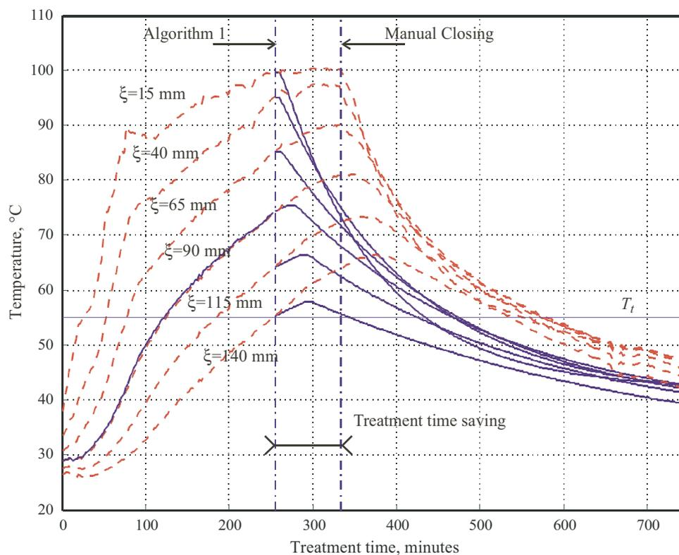
Fig. 5. Temperature behaviour during treatment; (dotted red line) manually controlled treatment; (solid blue line) automatic controlled treatment. In order to guarantee the target temperature  $T_t$  for at least 75 min in the soil at all the depths  $\xi \in [\xi_{min}, \xi_{max}]$ , the manual treatment lasted 336 min. The use of the control Algorithm 1 allowed to save 78 min of treatments, i.e. about the 23% of the treatment time
