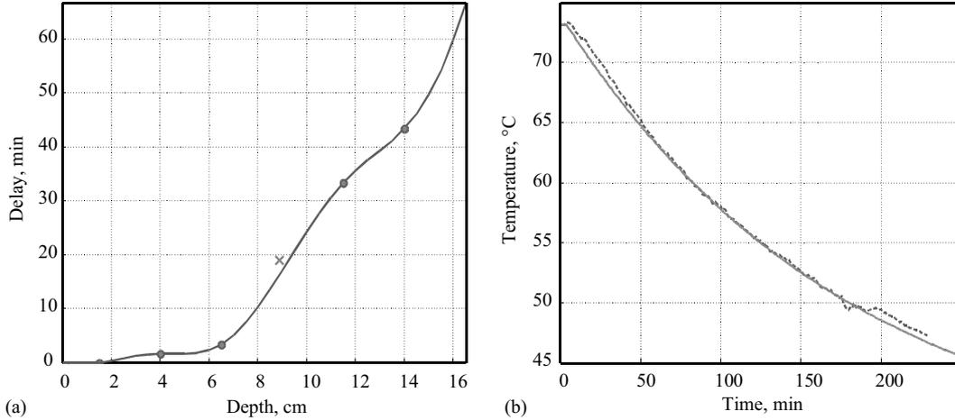
Fig. 4. (a) Behaviour of the input delay as a function of the depth:  $\times$ , measured delay at  $\xi=90$  mm; (b) validation of the linear parameter varying cooling subsystem, measured (dashed blue line) and simulated (solid red line) data for  $\xi=90$  mm
