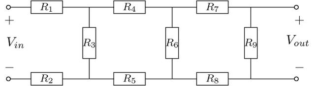
Fig. 5. Three-loop resistive ladder network.
