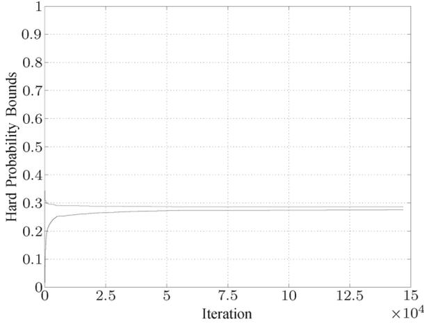
Fig. 7. Hard upper and lower bounds on the probability of stability for Example VII-C.
