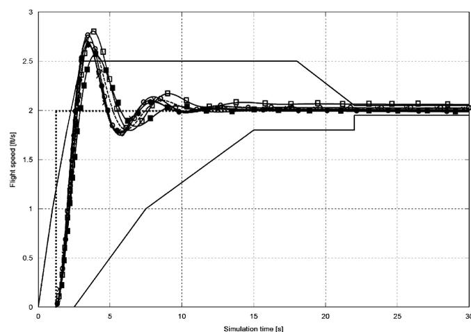
Fig. 5. Time domain response: flight speed command (black—reference; filled circle— $K^1$ ; empty square— $K^2$ ; cross— $K^3$ ; filled square— $K^4$ ; empty circle— $K^5$ ; dashed black— $K^{RP}$ ).
