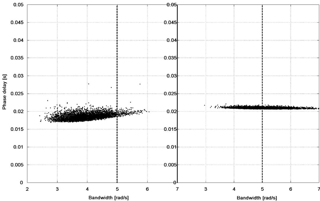
Fig. 4. Bandwidth criterion plot for  $K^5$  (left) and  $K^{PP}$  (right) highlighting the regions of interest for performance robustness analysis.
