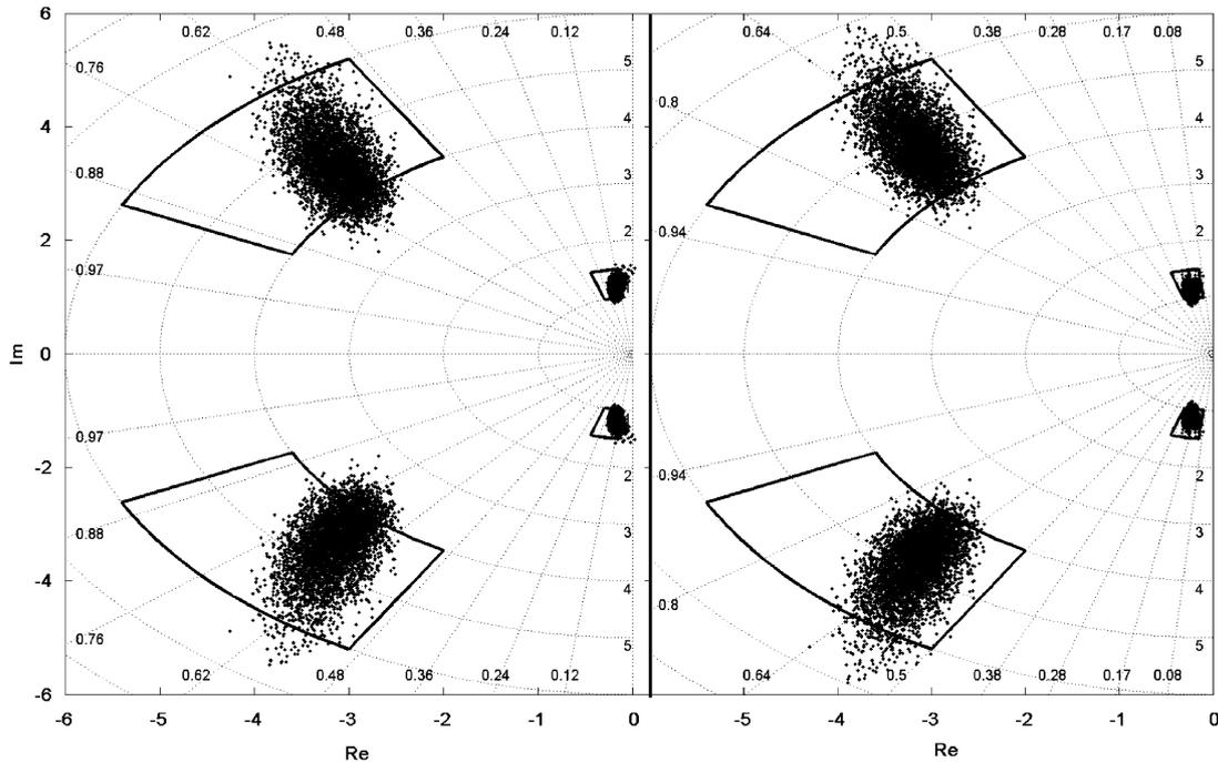
Fig. 3. Root locus plot for  $K^2$  (left) and  $K^4$  (right) highlighting the regions of interest for stability robustness analysis.
