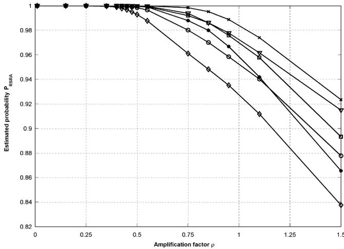
Fig. 1. Probability degradation function obtained with Algorithm RSRA ( $K^1$ —circle;  $K^2$ —asterisk;  $K^3$ —square;  $K^4$ —cross;  $K^5$ —diamond;  $K^{PP}$ —triangle).
