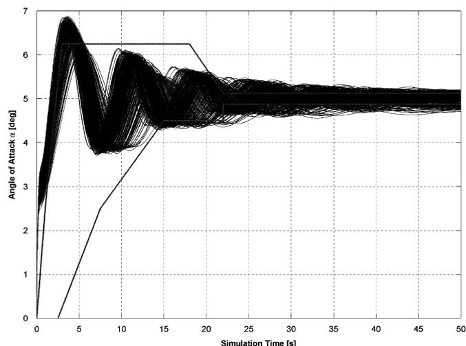
Fig. 6. Time domain response: angle-of-attack command (for  $N_A = 500$  uncertain systems).
